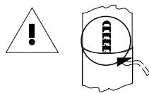
The scale must be readily legible and assembled such that it is facing the user's side.
